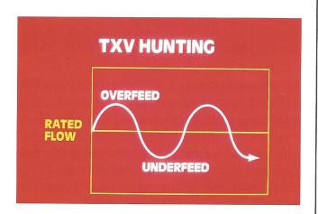
49. An oversized expansion valve will cause hunting, and hunting causes intermittent flooding, and starving of the evaporator, leading to possible damage resulting from the flooding itself, or from the potential flooded-starts and slugging it can create. This is especially true under light loads. In general, it is considered good practice to undersize rather than oversize an expansion valve.
