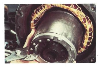
98. Next, remove the rotor from the compressor housing being careful not to damage the stator windings during disassembly. Any damage at disassembly will lead to a false analysis of the real problem.
