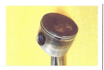
64. High discharge temperatures can cause worn or seized pistons, and piston rings, scored cylinder walls, and excessive wear on the wrist pin and pin bores.
