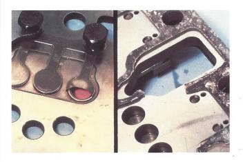
20. When a discharge valve has failed or a cylinder head gasket has blown, the pressure on top of the piston remains high and the bottom of the wrist pin never gets lubricated. The friction causes the bottom of the wrist pin hole (bore) to wear.
