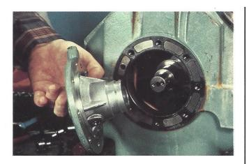
91. Oil pump and bearing failures are rare since they are the first components to get oil. However, they are also the first components to see any system contamination. When examining the bearing for scratches, do not confuse abnormal marks with normal machining marks. Remove the oil pump cover from the compressor housing. After removing the oil pump cover, it is a good idea to rotate the compressor using an Allen wrench to see if the pistons move with normal resistance.
