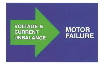
72. Electrical problems can also lead to compressor failure. In a three-phase compressor, motor failure can happen because of voltage and/or current unbalance. These are two types of problems which cause an increase in temperature that may go unnoticed for a long period of time.
