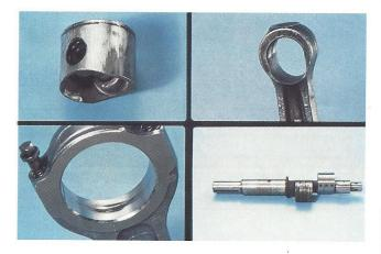
16. Loss of lubrication can cause the kinds of problems illustrated here.
