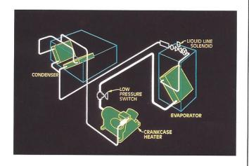
22. Another situation that leads to lubrication problems for compressors is refrigerant accumulation in the crankcase. When a compressor is started in this condition, the oil and refrigerant rapidly (violently) leave the compressor, creating a slug and a loss of lubrication.
