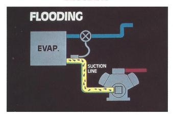
31. Another cause of compressor failure is flooding. Flooding is the **continuous** return of liquid refrigerant or liquid droplets in the suction vapor returning to the compressor during operation. It is usually associated with improper refrigerant flow control.
