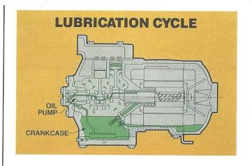
17. Proper lubrication is essential to the life of a compressor. To better understand how important this is, let's look at how the internal parts of the compressor are lubricated.
