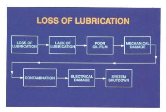
30. The chain of events resulting from a lack of lubrication leads to poor oil film coverage of wearing parts, mechanical damage, contamination leading to electrical damage and finally system shutdown.
