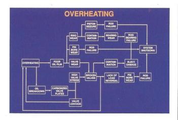
71. Overheating leads to thin oil and the resulting problems of accelerated wear. Severe overheating causes the oil to carbonize and contaminate. The resulting lubrication and contamination problems lead to mechanical damage and system shutdown.
