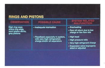
94. Extensive ring wear with sharp edges, and grey, discolored pistons usually are caused by poor lubrication due to refrigerant floodback. High compression ratio and discharge temperature will also cause accelerated piston and ring wear, but signs of overheating, such as discolored valves and valve plates, and pistons, are usually evident. Heavy suction valve wear will usually be evident if high discharge temperatures caused piston and ring wear.
