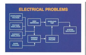
80. Electrical problems are usually caused by an electric supply imbalance or rapid compressor onoff cycling. All four typical electrical problems can lead to overheating and eventual burnout. In addition, rapid cycling can cause failure of the motor windings due to constant flexing of insulated turns and connections.
