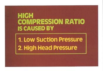
68. High compression ratio is caused by low suction pressure and high discharge pressure, or a combination of both.
