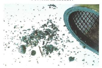
51. Contamination is another cause of compressor wear and failure. Contaminants are any substance or material other than the specified refrigerant and compressor oil, which cause a chemical reaction, or change the chemical composition of materials within the system.
