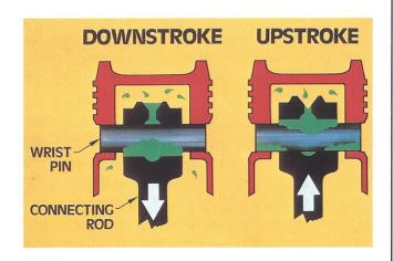
19. This is the connecting rod and wrist pin in cross section with clearances exaggerated for illustration.
