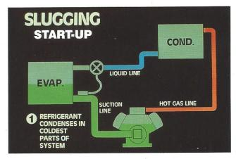
47. As described earlier, slugging is the return of a large quantity of liquid refrigerant or oil to the compressor. Refrigerant can condense during off cycles within any part of the system where temperatures become cold enough. This could be the evaporator coil, cooler, or compressor crankcase. On the next start-up, this liquid would find its way to the compressor cylinders as a slug the same way it does during a flooded start condition.
