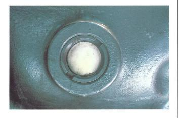
32. The result of flooding is usually oil dilution, which results in crankcase foaming, a cold compressor and conditions which are ideal for liquid refrigerant accumulation in the crankcase.
