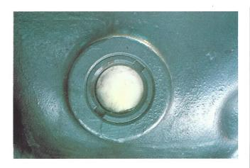
24. Loss of lubrication is also caused by oil leaving the compressor at excessive rates. This rapid loss of oil is usually associated with oil foaming which is easily observed in the compressor sight glass. If oil leaves the compressor at an excessive rate, it is not likely to be returned at the same rate.
