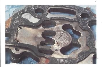
40. When parts, such as a suction valve break, the pieces may enter the cylinder. The clearance volume designed into the cylinder is not large enough to handle this "extra" material between the piston and valve plate.
