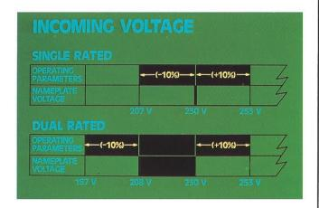
77. Another cause of overheating is too high or too low an incoming voltage. This is where the voltage is outside the maximum-minimum limits set by the manufacturer of the equipment. For a compressor with single rating of 230 volts, the operating limits are within  $\pm 10\%$  of 230 volts (207 to 253V).
