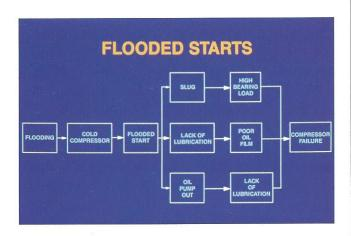
38. Floodback to a running compressor causes an abnormally cold crankcase which leads to liquid migration at shutdown. This causes flooded starts resulting in severe pressure in the cylinder (slugging). This causes severe overload to valves, gaskets, and bearings occurring at a time of marginal lubrication. The usual result is component failure.
