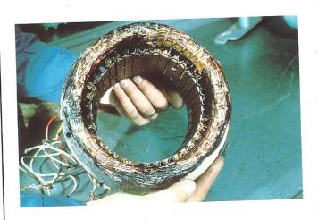
76. When a three-phase motor single phases, one phase is unaffected but the others generally show signs of overheating. The pattern of failure shows up in this slide. One phase is bright and shiny and clearly unaffected. This was the open phase. The other two phases are burned.
