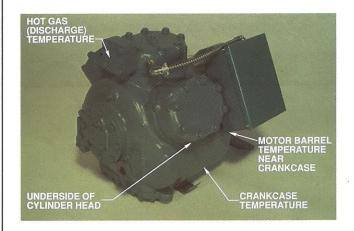
59. As mentioned previously, compressors are designed to handle normal thermal temperature gains, but when they operate outside design parameters, reduced life expectancy and potential damage result.
