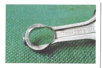
21. The resulting damage looks like this. Because of this, the compressor will operate hotter than normal, the noise level will increase and the compressor will have a rattling sound. This wear contributes to problems on other components such as rods, cylinder walls, and bearing surfaces as well. This type of damage generally goes unnoticed until it can be heard.
