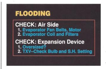
33. Air side problems are known to be a significant cause of flooding. These problems include broken evaporator fan belts, bad fan motors, dirty coils, and dirty filters. Although not often thought of as a real problem, their association with compressor failures is significant.
