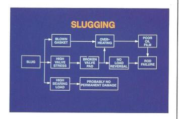
50. Slugging can lead to a blown gasket, high valve stress or high bearing loads. A blown gasket results in overheating, poor oil film cover-
