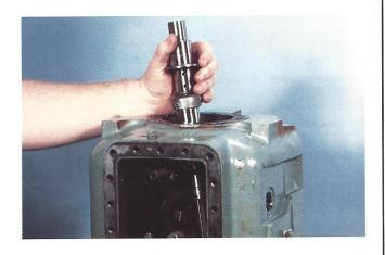
96. The next step is to remove the shaft from the compressor housing.
