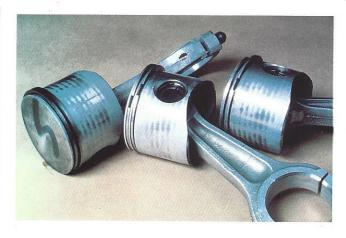
29. When inadequate cylinder bore lubrication takes place, discolored (grey) pistons, worn rings, and worn pistons result. This lack of lubrication is most frequently associated with lack of oil return during loss of charge or unloaded operating conditions, high but not necessarily extreme discharge temperatures due to loss of charge, or extreme floodback similar to what might be seen in split systems with large refrigerant charges.
