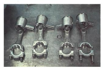
93. The pistons and connecting rods are removed from the cylinders and examined closely.
