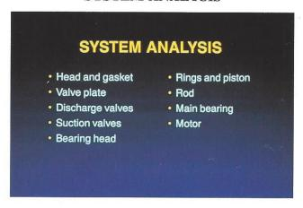
85. The first step in compressor and system analysis is to inspect the compressor. You may follow any orderly procedure to do this.
