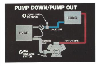
48. As mentioned earlier in the program, one method of minimizing refrigerant accumulation in the compressor is to incorporate a "single pumpout" control system. In this system a solenoid valve can be installed in the liquid line to prevent refrigerant flow to the evaporator. The thermostat operates the solenoid valve. The compressor pumps down the system and a low pressure switch stops the compressor after the refrigerant has been removed from the low side of the system.
