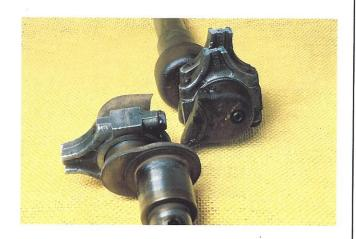
42. Liquid slugging can also have this disastrous effect. The connecting rods and even the crankshaft can break if the slug is significant enough. This type of failure would normally be caused by a tremendous slug at start-up.
