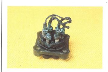
56. Moisture, as a contaminant has two primary detrimental effects. First, it will react with the refrigerant to form acid; and second, it could cause
