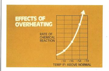
60. Laboratory tests show that with each 18° F rise in discharge temperature above normal, the chemical reaction rate between refrigerant and moisture, acid and oxides, acid and oil, and refrigerant and oil doubles. Doubling the chemical reaction very quickly begins to damage the compressor. The harmful effects of the acids, however, do not just limit themselves to the compressor, but can cause harm to the entire system.
