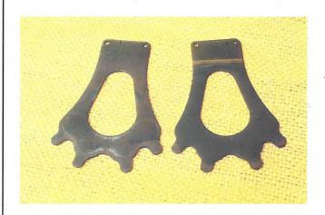
67. One component which suffers accelerated wear from the effects of high discharge pressures and temperatures is the suction valve. On the left you can see the outline of the suction port, which has worn into the valve. This wear has a tendency to stress the valve, making it more susceptible to failure.
