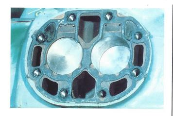
41. A blown cylinder head gasket or valve plate gasket may also indicate a liquid slug. The gasket will blow on an internal partition between the high and low side of the head. If the compressor remained running, the particular head where the failure occurred would run hot compared to the others. Feel the underside of the suspected cylinder head for unusually warm temperatures.
