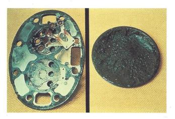
66. When the discharge line temperature approaches 300° F, system ingredients begin to break down. Oil will form sludge, which will coat the internal surfaces of the compressor with carbon as shown on the valve plate above. This sludge formation will collect in the oil pick-up screen in the compressor sump. This restriction makes proper lubrication nearly impossible. Damage under these circumstances is assured.
