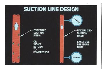
27. With regard to oil return and loss of lubrication, the design and installation of the suction line is the most critical line in the entire system. If a suction line is oversized, there will not be enough velocity to return the oil to the compressor. If undersized, there will be an excessive pressure drop in the line resulting in loss of capacity and an increase in superheat at the compressor.
