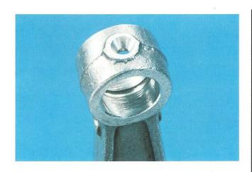
18. The wrist (piston) pin is lubricated by the refrigerant oil-vapor atmosphere (mist) in the crankcase. Oil collects on the different surfaces and components within the crankcase and lubricates them.
