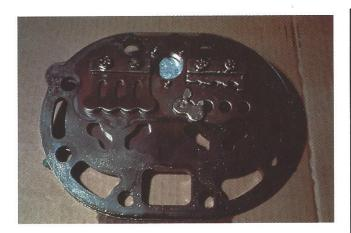
45. Long term, repeated mild slugging will cause metal fatigue of internal and external parts, for example, discharge lines and valve stops.
