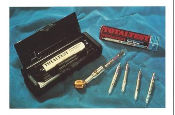
57. The oil in the compressor can be a dangerous substance as a result of acids. Compressor oil, although it may appear clear, should be tested for acidity. Use TOTALTEST® when contamination is suspected. This is especially true in the case of a compressor burn out.
