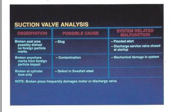
90. Suction valves will show damage similar to discharge valves.
