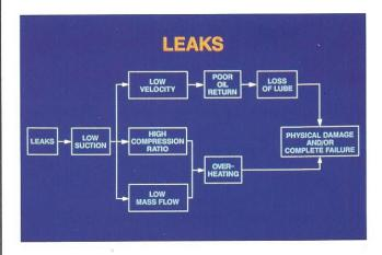
70. Leaks within the system can also lead to overheating. As refrigerant is lost, suction pressure will decrease causing lower refrigerant velocity, and lower mass flow, at the same time the compression ratio will increase.
