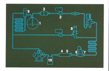
13. Receiver tanks (item 1) are often installed to compensate for variations in the system's refrigerant charge due to operating loads, and will temporarily compensate for minor refrigerant leaks.
