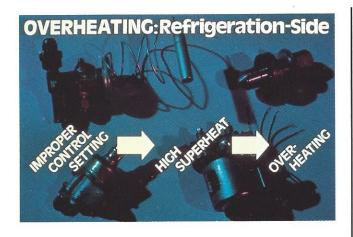
61. Reasons for overheating can be grouped into two basic categories: air-conditioning/refrigeration and electrical. On the A/C and refrigeration side, one of the most common causes of overheating is the improper setting of controls.
