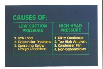
69. Low suction pressure is the most likely cause of high compression ratios. Low suction pressure is caused by low load, evaporator coil problems, air flow problems, partial loss of charge, improper pressure switch settings, frosted coil, or by operating the compressor below design conditions.
