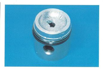
43. The force that results when a compressor tries to compress liquid refrigerant or oil is tremendous. Pressures of well over a thousand psi can be reached in the cylinder.
