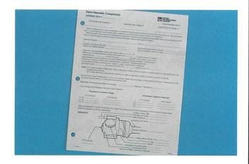
100. If it becomes necessary to call for assistance, be sure to have specific data such as compressor model and serial number, and system operating pressures and temperatures available before making the call. This information is necessary to effectively make a diagnosis.
