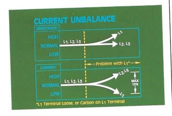
75. Voltage unbalance will cause a current unbalance but a current unbalance does not mean that a voltage unbalance necessarily exists. Take a three-phase situation where there is a loose terminal connection on one leg or where there is a buildup
