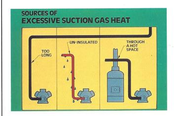
63. Bear in mind that heat is added to the suction gas as it flows from the evaporator to the compressor. The amount of heat can be excessive if the suction line is too long, uninsulated, or runs through a hot space, such as an equipment room.
