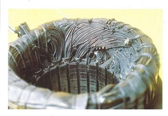
79. Finally, one of the causes of overheating often overlooked as a cause of compressor failure is rapid cycling. The start-stop cycling of controls and safety devices can result in shorted motor windings. Here is how it can happen:
