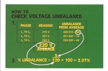
74. To check voltage unbalance take the voltage readings between phases at the disconnect or the compressor contactor while the compressor is operating.
