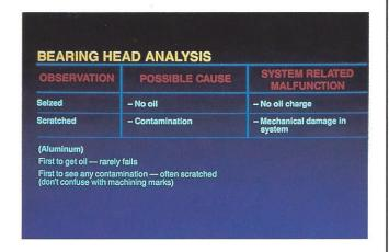
92. Bearing head analysis will indicate either a seized or scratched bearing surface as a malfunction. Again, do not confuse normal machining marks with scratches due to contamination.
