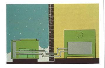
10. Split system applications present an additional set of problems. Compressors in these systems must deal with piping considerations, improper mixing and matching of components, additional oil return problems, duct work considerations, and ambient temperature variations.
