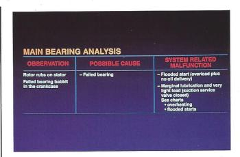
97. Indication of bearing failure such as the rotor rubbing on the stator is commonly caused in compressors by flooded start conditions.
