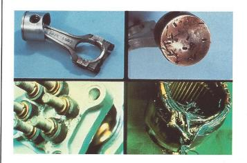
3. The system and service related failures continue to show evidence of electrical or mechanical failure. These include broken valves, scored shafts, broken rods, and overheating. Electrical failures include single phasing, overheating, and
